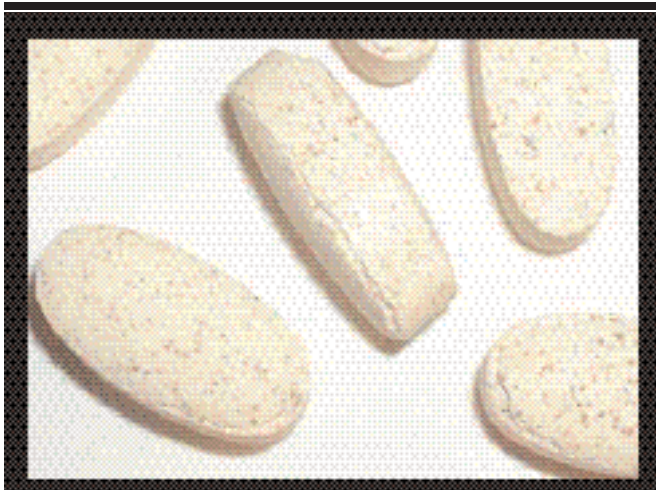
Figure 5: The top of this tablet is coming off the rest of the tablet. This is called capping .
