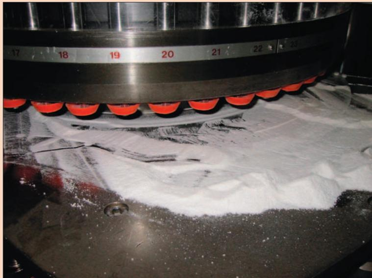
replace it as needed. When the blade is in bad condition or set up incorrectly, it won't scrape the die table clean, and you'll have problems with weight control.
