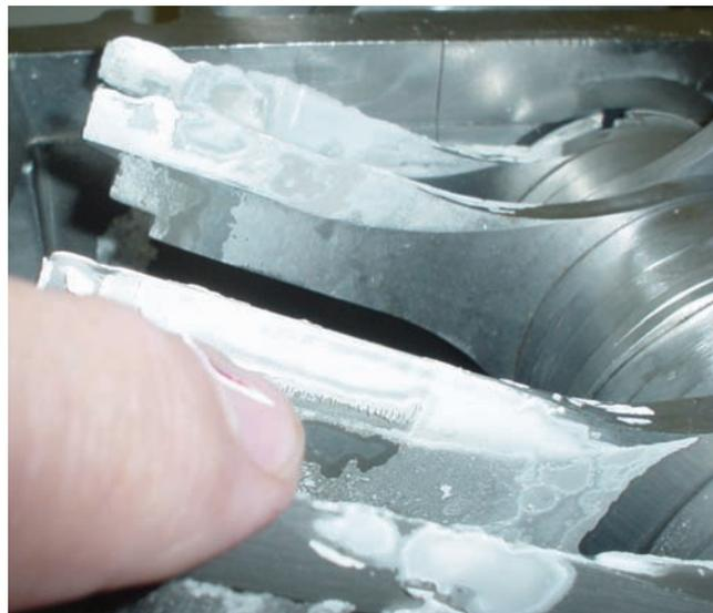
Photo shows wet, densified buildup on the blades of a mill used before final blending and tableting. If the tablet operators knew about this buildup, they could anticipate the picking and sticking that is likely to ensue. But usually, they aren't privy to information about upstream processes.
