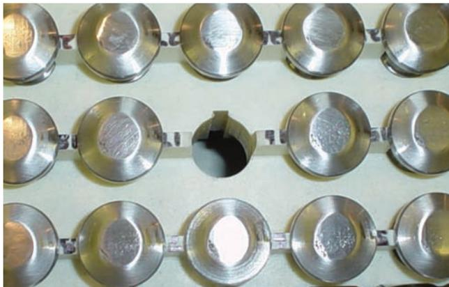
Damaged tooling is the result of tight punches caused by poorly processed powders. Don't blame the press operator. It more likely stems from high compression forces, high ejection forces, poor lubrication, and/or a lack of dust collection. The tablet press is the report card, laying bare the mistakes of the previous operations.
