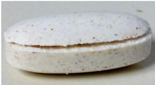
A capped tablet. Capping can occur when entrapped air is released from the tablet or as a result of the formulation's elastic properties.
