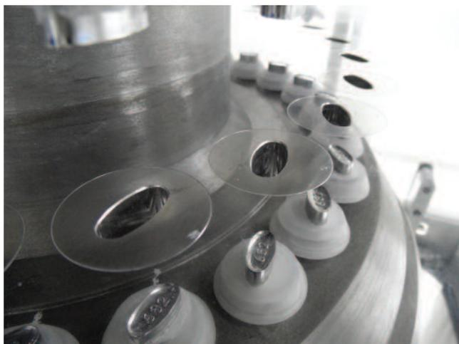
Embossed numbers on the punch face can pick the formulation from the tablet.
