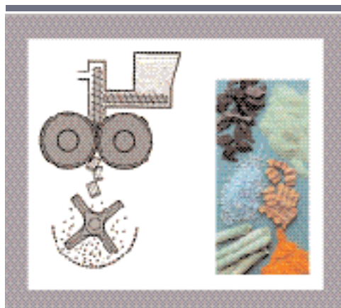
Figure 4: A chilsonator with mill (Fitzpatrick, Elmhurst, IL).
