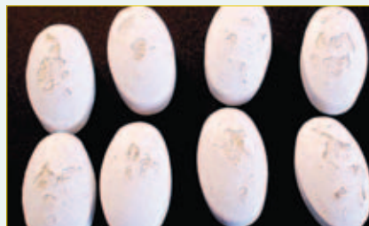
I attribute the peeling in this photo to excessive moisture within the tablet, which prevented the coating from adhering. However, the tablet coating also pulled the granulation out of the tablet, a picking defect. That is usually caused by over-wetting the tablet or by a tablet that is too soft.
