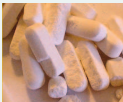
Just one broken tablet can distribute particles to all the other tablets and mar their appearance. These tablets likely broke because they had poor hardness.
