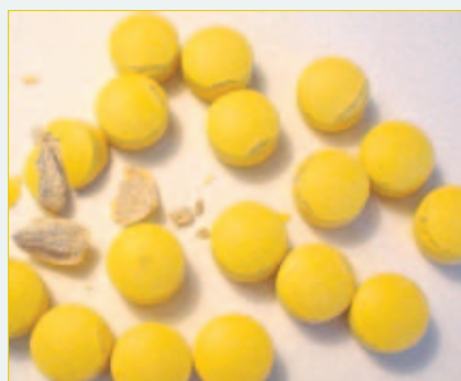
This photo shows multiple defects. The initial problem was erosion of the tablet edge due to a soft or friable tablet or because the pan was turning too fast or both. Peeling and breakage also appear here.
