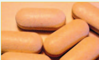
This photo shows a very porous tablet that prevented the coating from adhering to the surface. These tablets should have been coated longer, and the atomization pressure should have been reduced to decrease the slight orange peel, or textured, surface.
