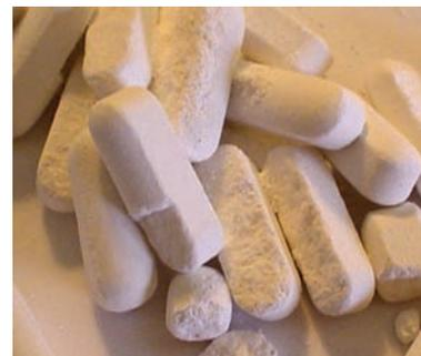
*These broken tablets are the result of poor compressibility.*
