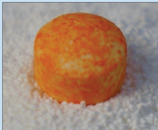
a. A mottled tablet indicates that the tablet was too soft and eroded and/or that the coating process was too wet.
