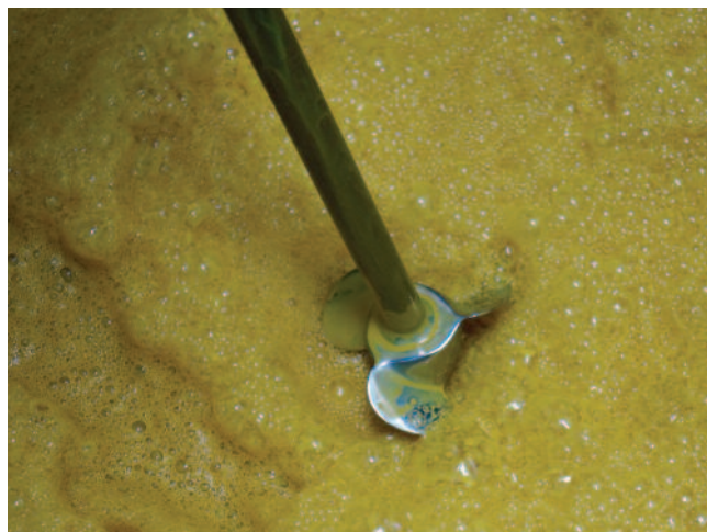
Avoid introducing air when you prepare coatings. This suspension is too foamy.
