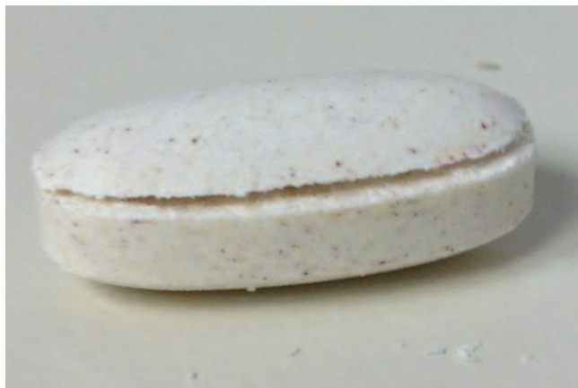
A capped tablet. This reject should never enter the coating drum. Sometimes the heat of the coating process will cause acceptable tablets to cap.
