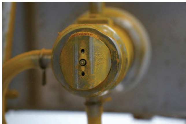
Buildup on nozzles can flake, enter the tablet bed, and cause a defect called picking.
