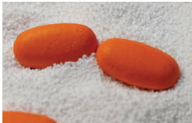
The erosion visible beneath the coating occurred during the preheat cycle, which should have been stopped. Tablets with a soft surface are nearly impossible to coat without creating defects.
